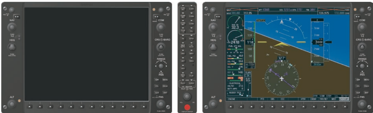
Figure 2.7.2 G1000 Reversionary Mode: Failed PFD
